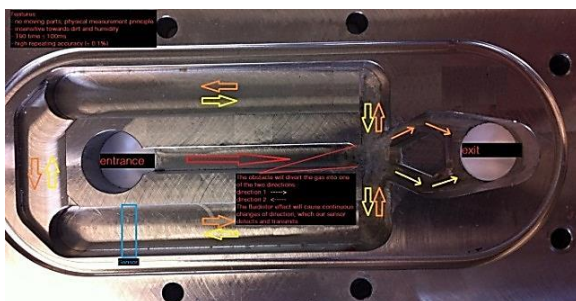
Oscillating Principle of Measurement
